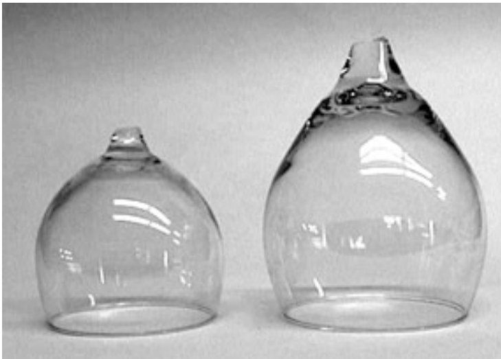
The globe on the right will show stronger lensing effects than the left globe.
