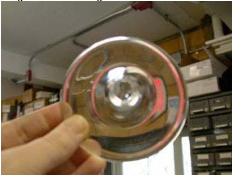
Note the distortion of red EXIT sign around the curve of the glass.
